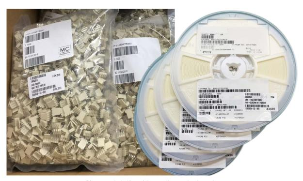
Picture 6: Labelling of the smallest packaging unit
