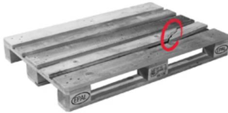
A board is broken crosswise or diagonally.
