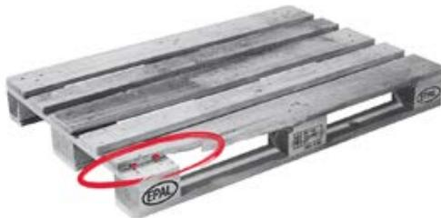
A bottom or cover board that is splintered in such a way that more than one nail or screw shaft is visible.
